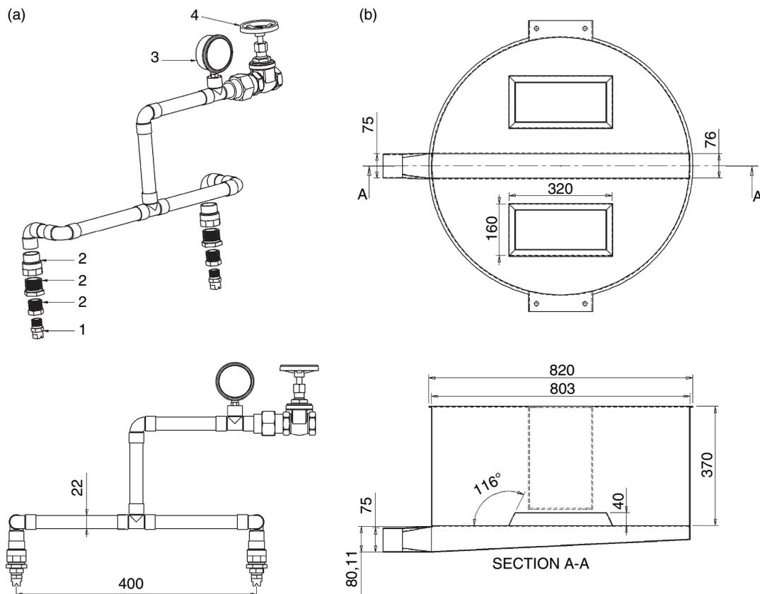
**Figure 4** (a) Details of the water application unit: (1) nozzles Veejet; (2) connections; (3) water pressure gauge; (4) manual valve and (b) blocking device for intercepting water. Units in mm.
