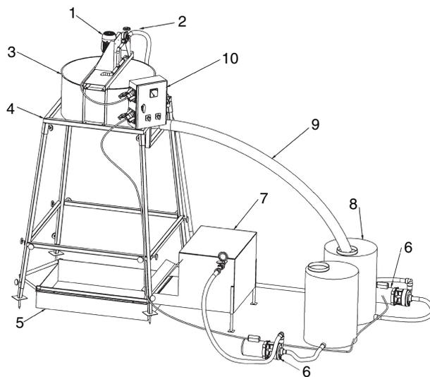
**Figure 1** General view of *InfiAsper2*, integrated rainfall and overland flow simulator: (1) motor; (2) water application; (3) blocking device; (4) upper frame; (5) run-off collector; (6) water pump; (7) overland flow module; (8) tank; (9) excess water; (10) electric panel control.
