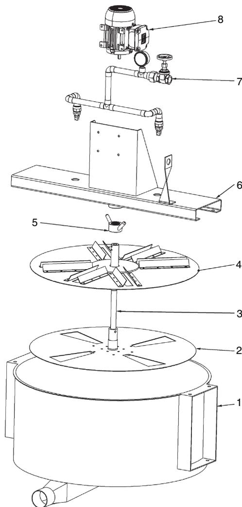
**Figure 3** Main elements of the water application unit of *InfiAsper2*. (1) blocking device for intercepting water; (2) lower disc; (3) axle; (4) upper disc; (5) nut; (6) support beam of rotating discs, water application system and motor; (7) water application unit; and (8) motor.
