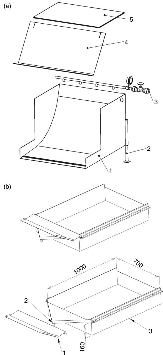
**Figure 6** (a) Overland flow applicator device: (1) lateral overland flow; (2) support legs with a levelling gadget; (3) water application unit; (4) front cover; (5) upper cover; and (b) run-off collector: (1) front cover; (2) collector point; (3) lateral delimiter. Units in mm.
