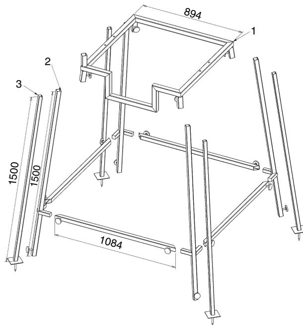
**Figure 2** Framework unit: (1) upper frame; (2) lower frame; and (3) telescopic system. Units in mm.
