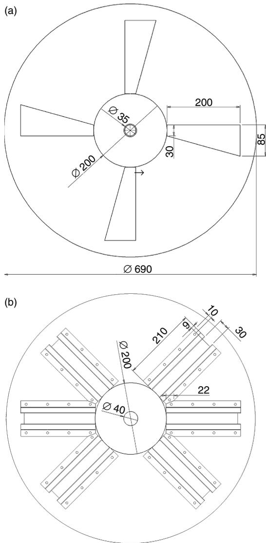
**Figure 5** Rotating shutter: (a) lower disk, and (b) upper disk. Units in mm.
