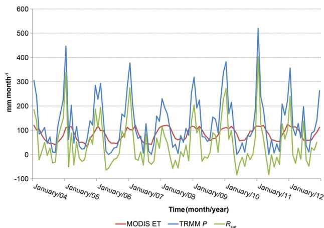
**Fig. 3** Monthly MOD16 evapotranspiration (ET), TRMM rainfall ( $P$ ) and groundwater recharge ( $R_{sat}$ ) over the 2004–2012 period. Negative values of  $R_{sat}$  indicated soil water deficit
